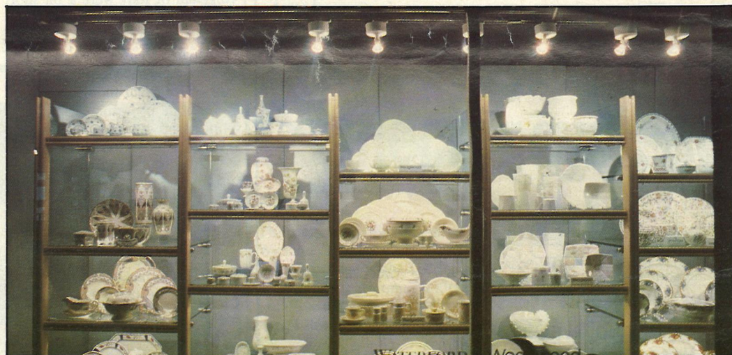
China displayed on glass shelving in a prime shopping site: Waterford/Wedgwood window at Oxford Circus, London, lit by Concord's low voltage Tiller spotlights on track and using 28° and 13° lamps.
