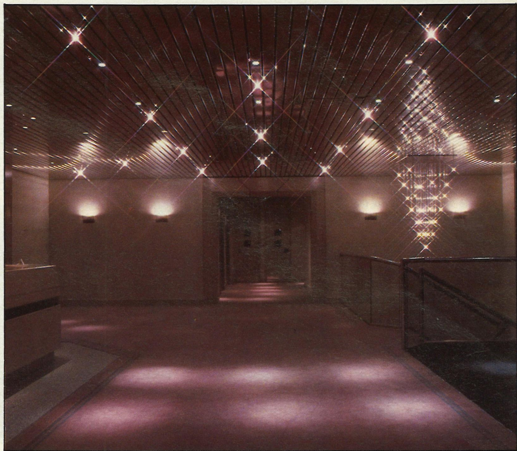
Left: entrance to a building on the Guildford Business Park, Surrey, lit by 150W metal halide projectors that give a punchy light on the floor.
